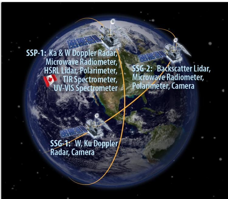
**Figure 1.2.** Summary of the final recommendation from the ACCP study indicating a single satellite in polar orbit and two satellites in an inclined orbit.
