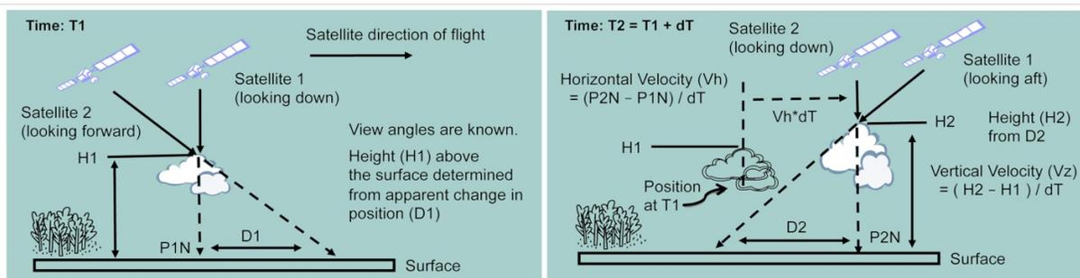
**Figure 7.9.** Illustration of tandem stereo imaging. Two view angles (one nadir and one forward or one aftward view) from tandem spacecraft provide instantaneous stereoscopic heights and time-lapse imagery for retrieval of cloud horizontal and vertical velocities. Figure courtesy of Roger Marchand, Univ. of Washington.
