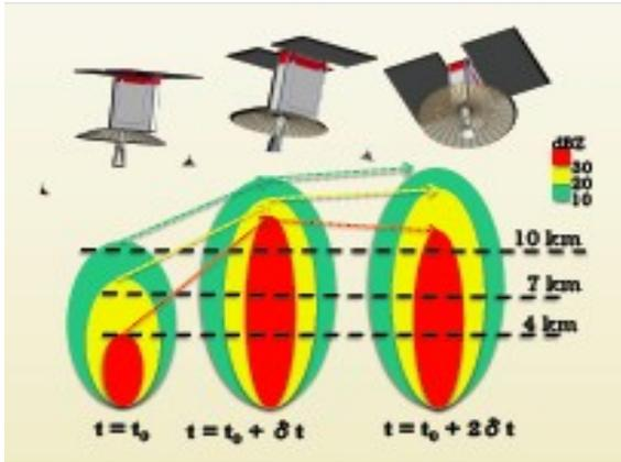
**Figure 7.14.** A schematic depiction of a three-satellite cluster observing a growing convective cloud. Each profile would be matched to the preceding profile collected  $dt$  seconds before it. One concept being considered is for  $dt=30$  and 90s. From Stephens et al. 2020.
