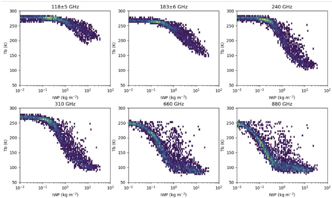
**Figure 8.6.** Brightness Temperature-Ice Water Path density plots for selected frequencies covering the range considered in ACCP candidate architectures. The wide dynamic range of IWP necessitates a wide range of frequencies reaching into the sub-mm range ( $> 600$  GHz) to achieve ACCP objectives regarding high cloud feedback. Figure provided courtesy of S. Joe Munchak (NASA GSFC, Munchak et al. 2020).
