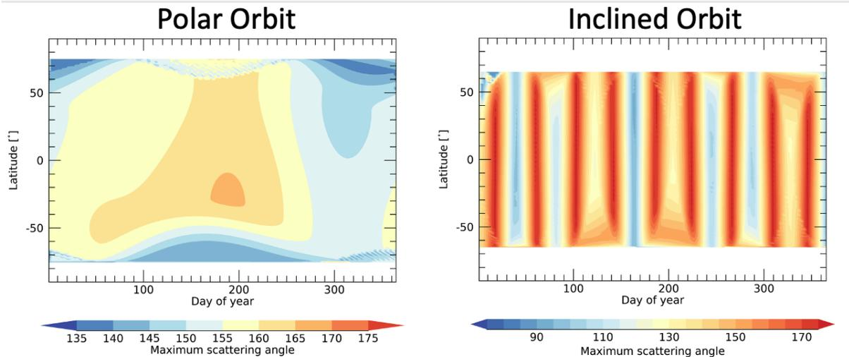
**Figure 8.5.** Maximum scattering angles available for use in polarimetry measurements for (left) polar and (right) inclined orbits. The maximum available information is obtained where the maximum scattering angle is large. These results were used to scale the polarimetry informed GV scores to account for sampling. Figure Courtesy Sebastian Van Dienenhoven (Columbia University and NASA GISS).
