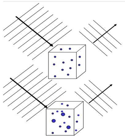
**Figure 7.3** A simple schematic of reflection by hypothetical volume of scatterers. The reflectivity at radar wavelengths varies with particle size ( $D$ ) approximately as  $D^6$ . When drops are all of the same size (upper), the reflectivity varies as the water content  $w^2 \sim (D^3)^2$ . For more realistic cloudy volumes (lower) composed of hydrometers of distributed sizes, the reflectivity no longer varies in a simple and non-unique way with water content.
