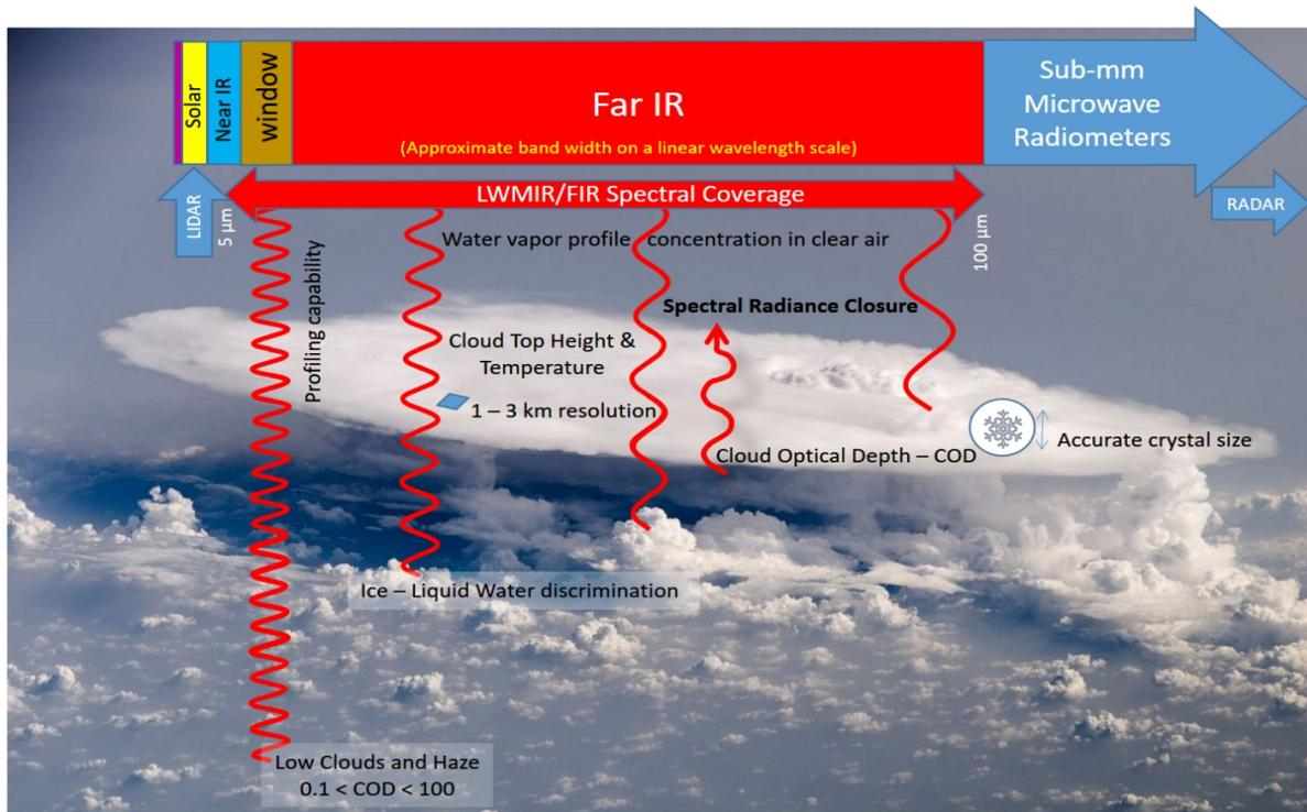
**Figure 7.8.** Spectral domain of LWMIR/FIR spectrometer bridging the critical gap of terrestrial emission at wavelengths between 5 and 100 $\mu\text{m}$ . Shorter thermal emission wavelengths in the atmospheric window are mostly transparent in clear sky, while longer wavelengths progressively reach higher altitudes, allowing for profiling. Labels show some of the key geophysical variables probed by the longwave spectrometer. (Cloud picture: NASA).
