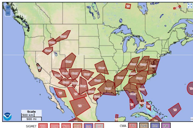
Figure 3.3.1. Example image from the Aviation Weather Center’s Significant Meteorological Information (SIGMET) map, showing large regions of turbulence and convection, primarily on CONUS. Credit: https://www.aviationweather.gov/sigmet
